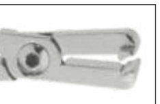
DI-1399 Detailing step plier double sided offset beak permits bayonet bends. Creates right hand or left hand step-up or stepdown at 1/2", 3/4" or 1mm increments.
